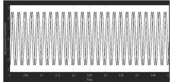
Fig.11. dq-Current Controller outputs of Multilevel Inverter Grid Tied System.
