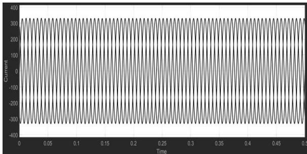
Fig.10. Current output of Multilevel Inverter Grid Tied System.
