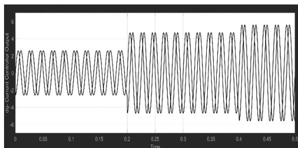
Fig.15. dq-Current Controller outputs of Multilevel Inverter Grid Tied System with 2 three phase faults.
