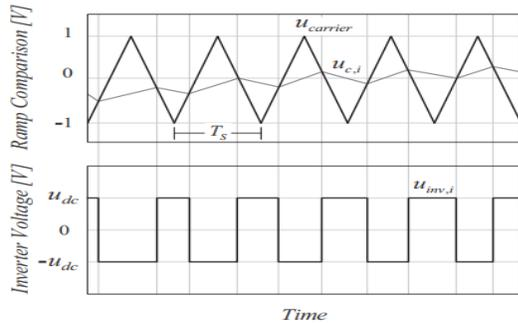
Fig.4. Output of Ramp Comparison Current Controller
