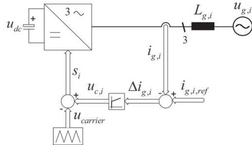
Fig.3. Ramp Comparison current controller
