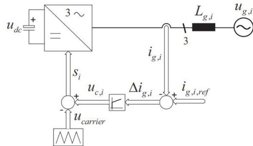
Fig.3. Ramp Comparison current controller
