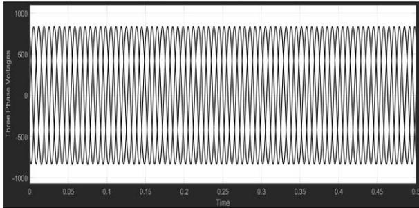
Fig.9. Voltage output of Multilevel Inverter Grid Tied System.
