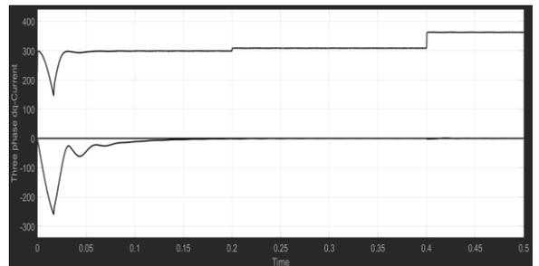
Fig.14. dq-Current outputs of Multilevel Inverter Grid Tied System with 2 Three phase faults.
