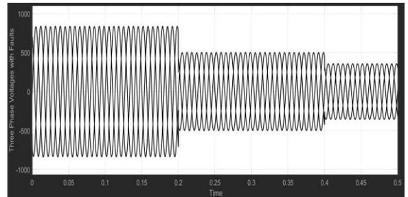
Fig.12. Voltage output of Multilevel Inverter Grid Tied System with 2 Three phase faults.
