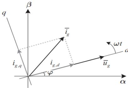
Fig.6. Dq reference frame aligned to grid voltage.
