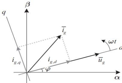
Fig.6. Dq reference frame aligned to grid voltage.
