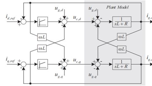
Fig.8. Voltage Oriented Current Controller with Decoupling and feedforward
