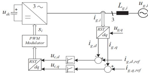
Fig.7. Voltage Oriented Current Controller.
