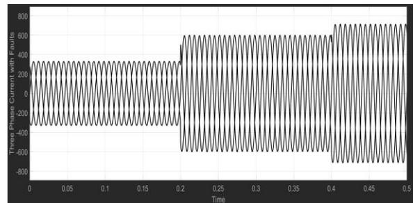
Fig.13. Current outputs of Multilevel Inverter Grid Tied System with 2 Three phase faults.
