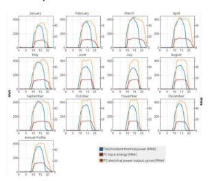
Fig. 6. Hourly data of PC thermal input, PC gross electrical output and Incident field thermal power for the plant
