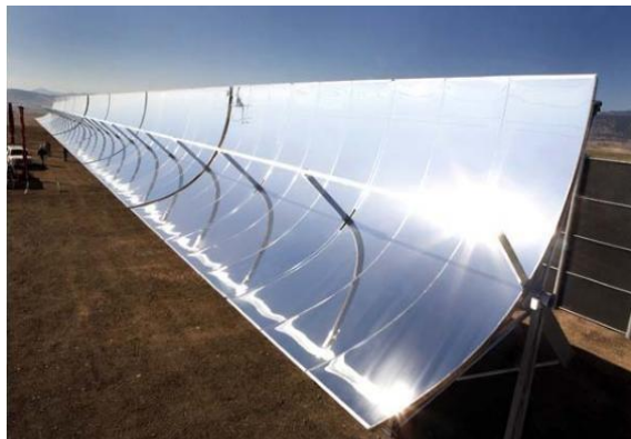
Fig. 6. Sky Fuel Parabolic Trough collector [13].
