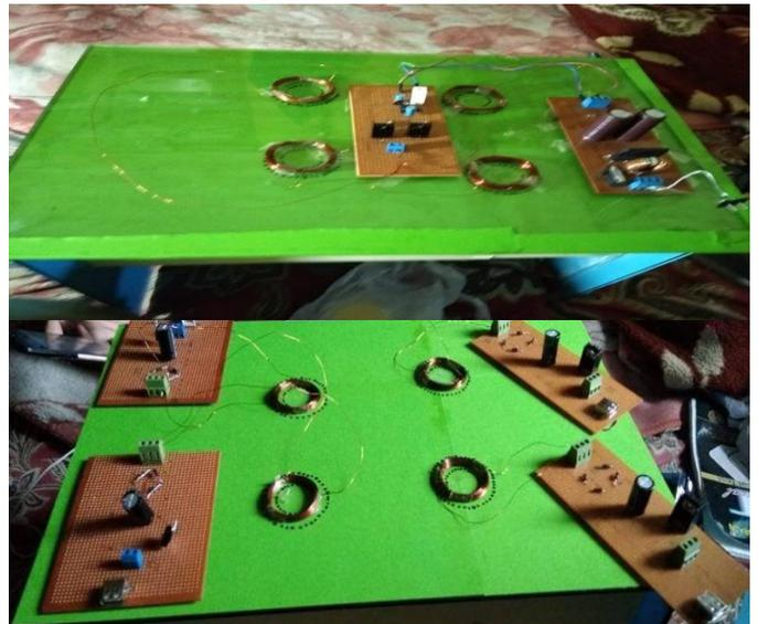
Figure 5: Hardware set up consisting of four receivers coils on the top of Table.
