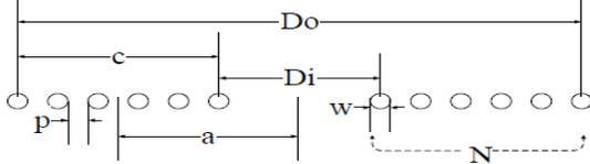
Figure 03. Cross sectional view of spiral flat coil
