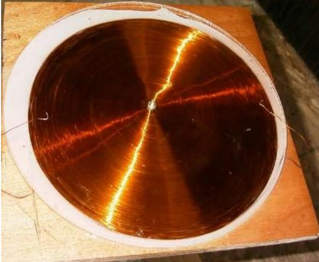
Figure 2 Spiral Coil consisting a number of turns
