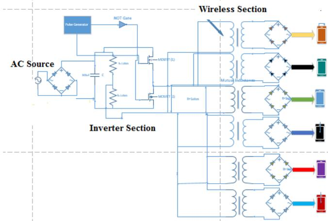
Figure:01 Theoretical Model of proposed multiple wireless charging inductive power transfer.
