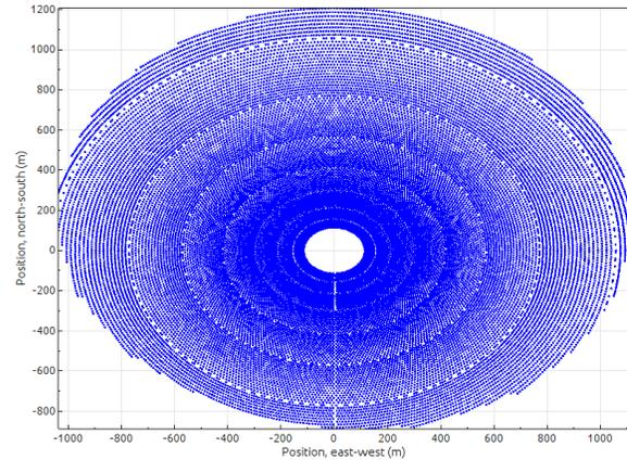
Fig 5: Heliostat Positioning
