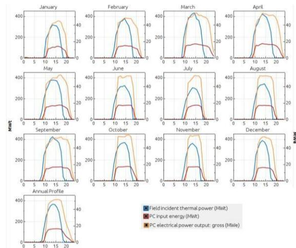
Fig. 6. Hourly data of PC thermal input, PC gross electrical output and Incident field thermal power for the plant
