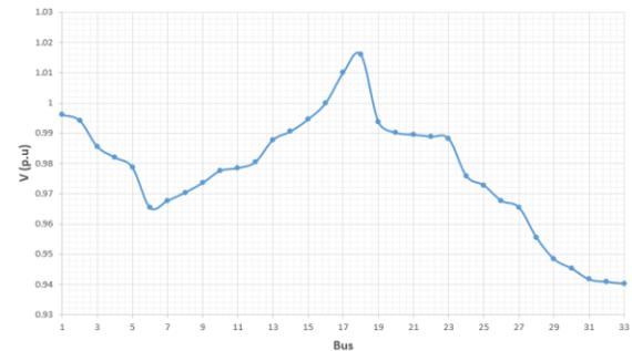
Fig.6. Bus voltages when PV is integrated at bus 18.
