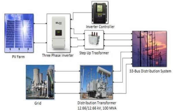
Fig.3. Complete model in Matlab/Simulink.
