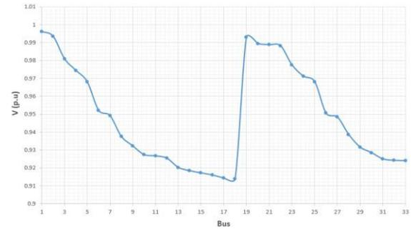
Fig.5. Bus voltages when no PV is integrated.
