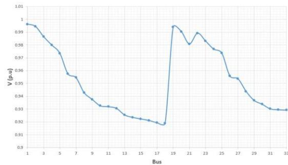
Fig.9. Bus voltages when PV is integrated at bus 3.
