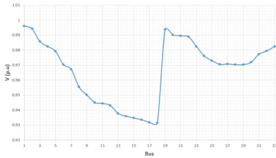
Fig.7. Bus voltages when PV is integrated at bus 33.
