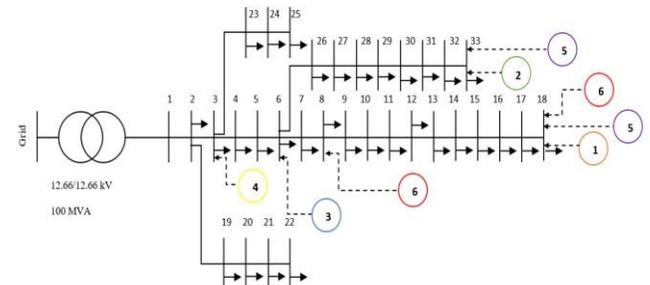
Fig.4. IEEE-33 Bus System with six different scenarios indicated.
