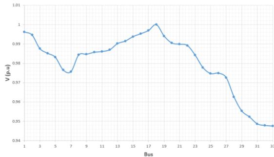
Fig.10. Bus voltages when PV is integrated at bus 18 and bus 8.
