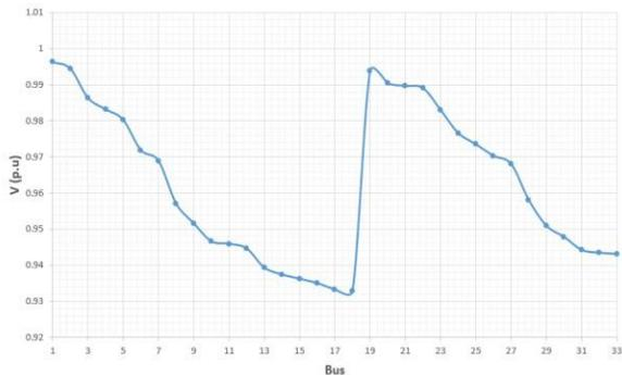
Fig.8. Bus voltages when PV is integrated at bus 6.
