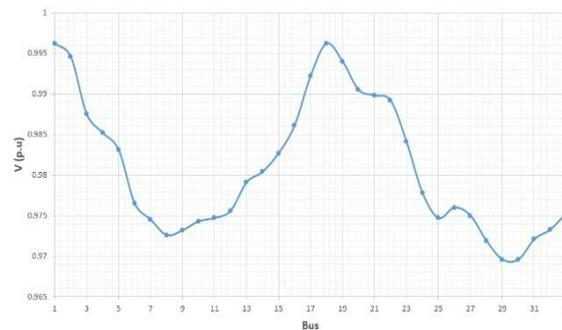
Fig.10. Bus voltages when PV is integrated at bus 33 and bus 18.
