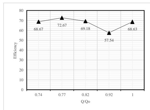
Fig 10: Efficiency Plot of 400 kW Kamri Astore HP Plant.
