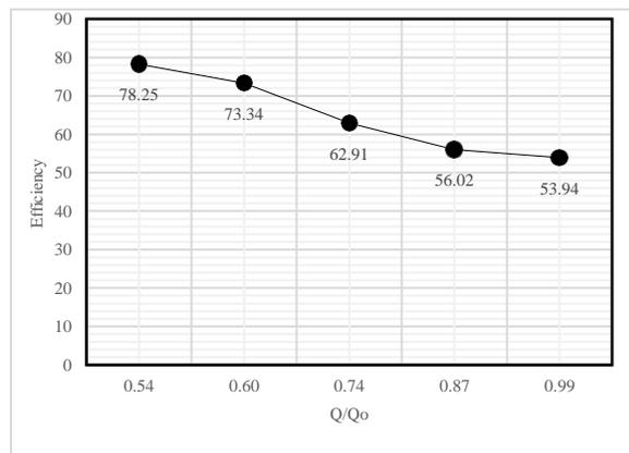
Fig 8: Efficiency Plot of 500 kW Sumayar Nagar HP Plant.
