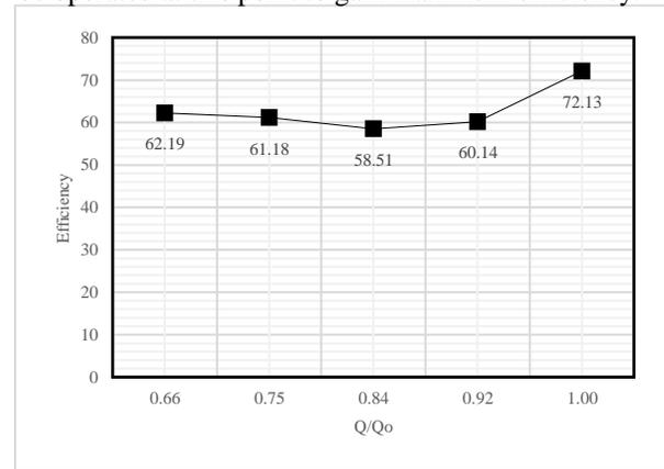
Fig 9: Efficiency Plot of 500 kW Chamugar Gilgit HP Plant.
