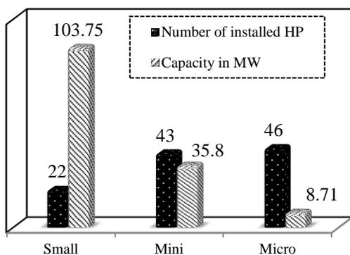
Fig 2: Hydel Plants categories and Installed Capacity in GB (data source: GBPWD/GIZ).
